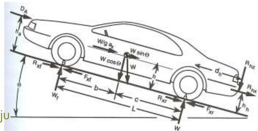
$$W_f = (W \cos \theta * c - R_{hx} * h_h - R_{hz} * d_h - \frac{W}{g} a_x * h - D_A * h_a - W \sin \theta * h) / L$$
